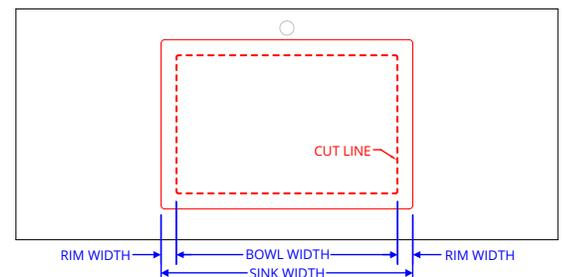
2. Measure the distance between the inside edge of the bowl and the outer edge of the rim. Mark the counter top inside of the first tracing. The distance between the two lines should be equal to the width of the rim. Cut the counter top along the inner line. Confirm a proper fit by temporarily placing sink under the cut-out.
