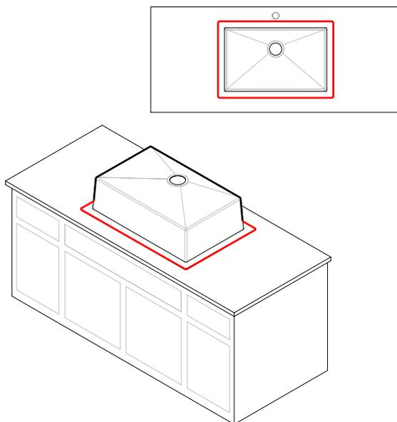
1. Place the basin of the sink upside down on the counter top surface and mark the surface of the counter top by tracing around the outside edge of the rim. Make sure to provide clearance for your faucet or any other fixtures (including clearance for full range of motion on all moving parts). Make sure to account for mounting studs and clips.
