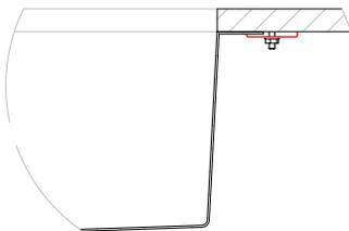
6. Confirm the basin is sitting level in all directions while pressing to seal. Remove all excess silicone.
