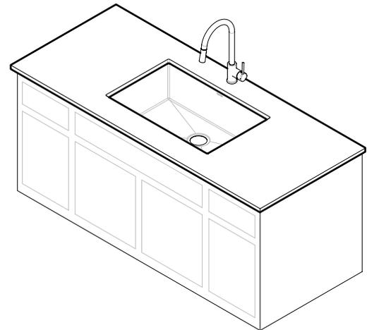
5. Position the sink under the counter top and secure it in place using mounting clip fasteners.
