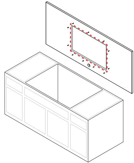
4. Apply 100% non-water-based silicone underneath the counter top around the cut-out area.
