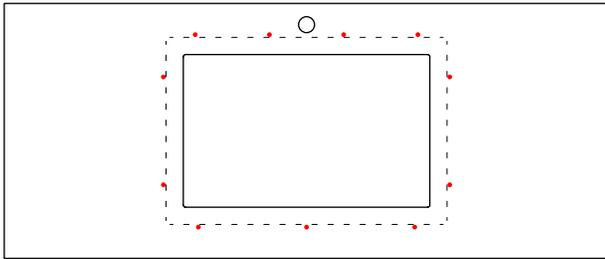
3. Install studs for mounting clips on the underside of the counter top, leaving sufficient clearance for the sink rim.
