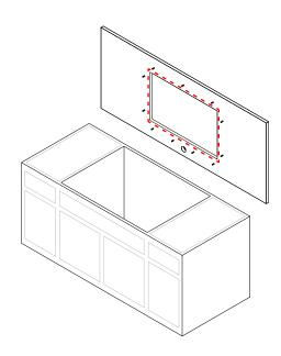
3. Install studs for mounting clips on the underside of the counter top, leaving sufficient clearance for the sink rim.
