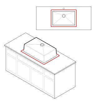
Place the basin of the sink upside down on the counter top surface and mark the surface of the counter top by tracing around the outside edge of the rim. Make sure to provide clearance for your faucet or any other fixtures (including clearance for full range of motion on all moving parts). Make sure to account for mounting studs and clips.
