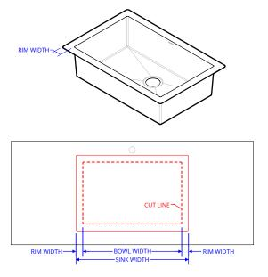
Measure the distance between the inside edge of the bowl and the outer edge of the rim. Mark the counter top inside of the first tracing. The distance between the two lines should be equal to the width of the rim. Cut the counter top along the inner line. Confirm a proper fit by temporarily placing sink under the cut-out.
