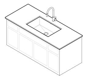
$5. \qquad \begin{array}{ll} \text{Position the sink under the counter top and secure it in place using} \\ \text{mounting clip fasteners.} \end{array}$
