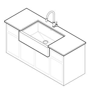
6. Position the counter top onto the cabinet and over the sink. Confirm the basin is sitting level in all directions while pressing to seal. Remove all excess silicone.
