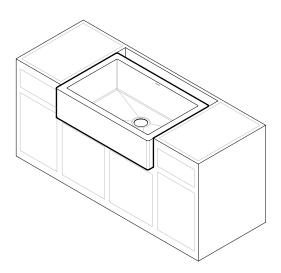
4. Place the sink into the opening of the support frame built in Step 1. The frame should support the entire weight of the sink. Confirm the sink is level in all directions and in-line with the top of the cabinet.
