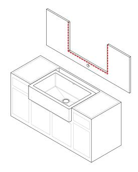
$5. \qquad \mbox{Apply 100\% non-water-based silicone underneath the counter top around the cut-out area.}$
