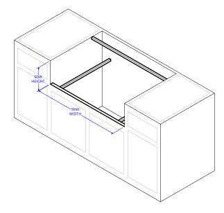
Build a support frame into the cabinet, or install support bars from the front to the back of the cabinet along the inner sides. The support should be positioned so the sink, when installed, is level and in-line with the top of the cabinet. If you are unsure about how to build a frame or install support bars that will provide adequate support, consult a professional installer.
